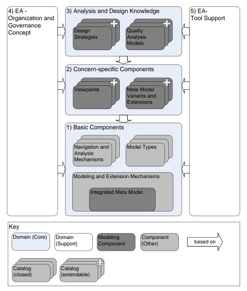
Figure 2: Top-level structure of the proposed engineering approach to EA design
